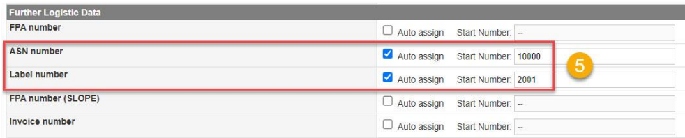
Figure 23 Company Administrator can define the auto assign of ASN and label number
