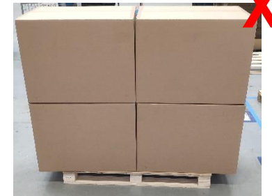
Not allowed – Up to 40% reduction in strength
