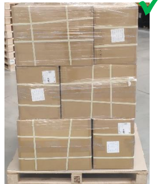
Still OK, but may result in a 33% structural weakness
